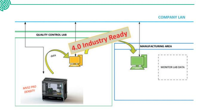
The system can be fully integrated within the company LAN with the ability to transfer analytical data to the areas of competence identified automatically.
