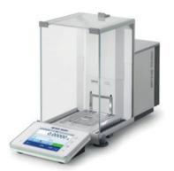
Analytical Electronic Balance with underplane support weight to position the support sample in the measurement area of the **MVS2pro**. The balance suggested is 5 decimal places in grams like: MS, XSR, XPR series (d= 0,01 mg). The Balance is directly controlled by **MVS2pro** via USB.
